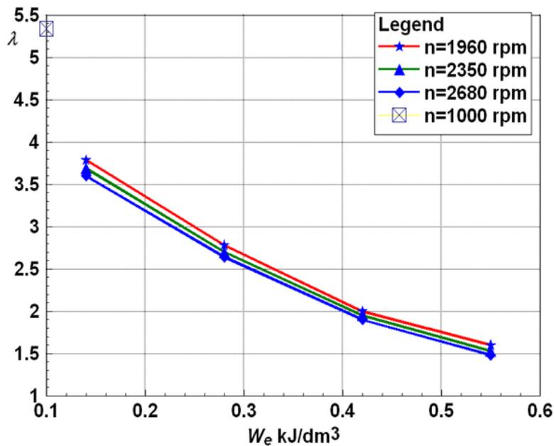
Figure 4. Working regimes of the engine and air excess ratio
