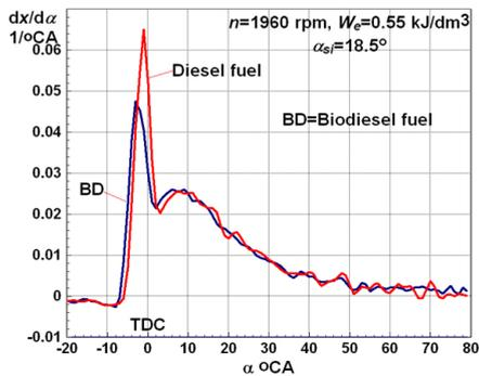
Figure 6. Actual normalized rate of heat release diagrams
