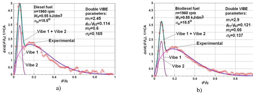
Figure 8. Approximation of two actual rate of heat release diagrams by a double Vibe function
