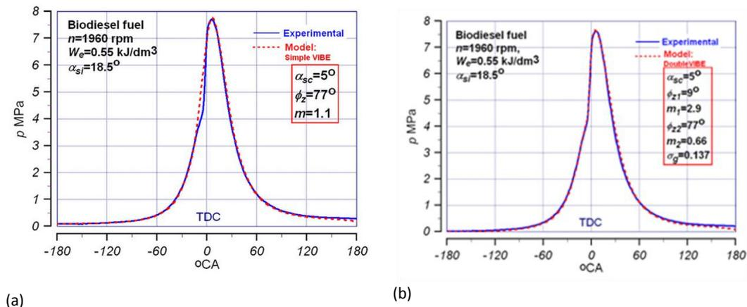
**Figure 1. Results of the model and experimental data of the indicator diagrams**
