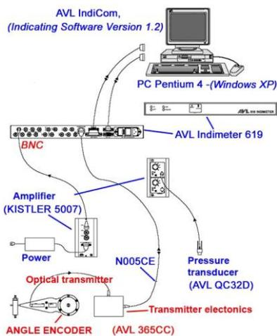
Figure 2. AVL Indicating system diagram
