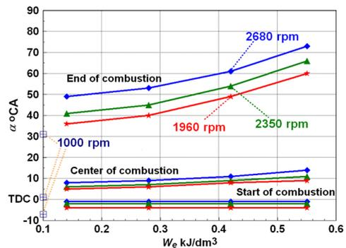
Figure 7. Start, centre and end of combustion while the engine works with biodiesel fuel
