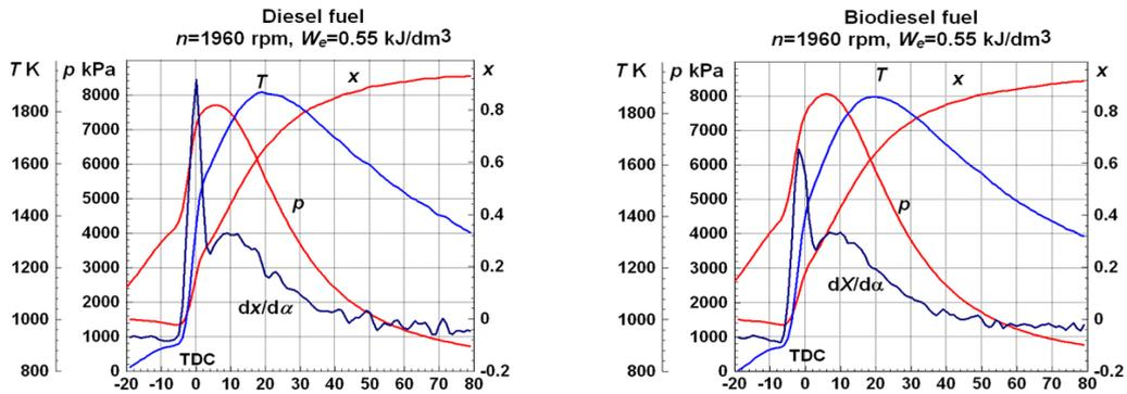
Figure 5. The results of pressure diagrams analysis: normalized rate of heat release  $dx/d\alpha$ , cumulative heat released  $x$ , and mean gas temperature  $T$
