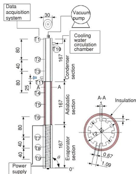
Figure 1. Experimental set-up
