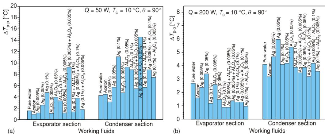
Figure 9. Effect of different working fluids on temperature fluctuation
