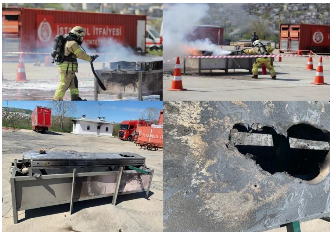
Figure 3. structural damage after the experiment and extinguishing operations performed during fire extinguishing
