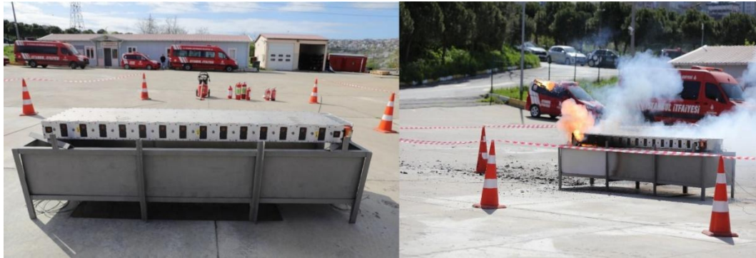
Figure 1. Battery on experiment table and fire start
