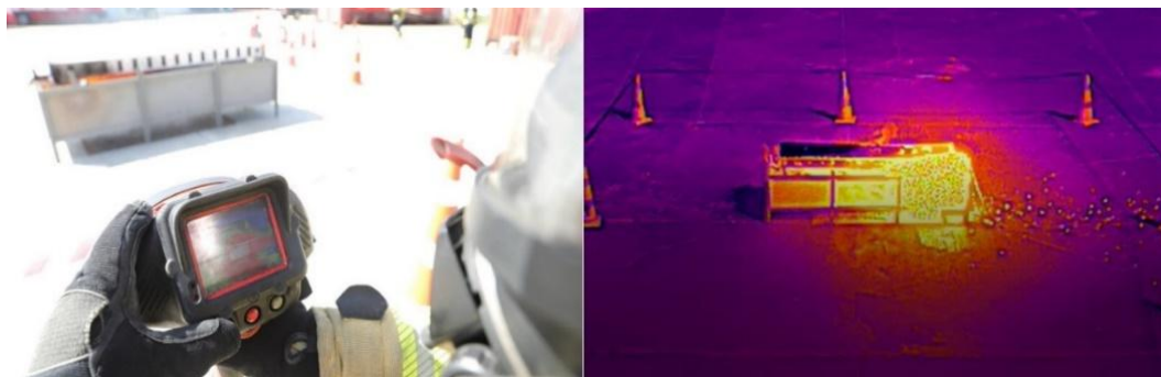
Figure 2. Battery fire test view under thermal camera
