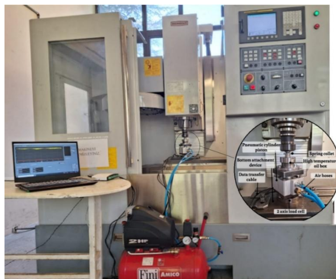
Figure 4. Image of the wear test set-up
