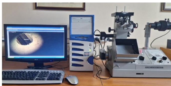
Figure 5. Optical microscope used to measure the ball wear trace diameter
