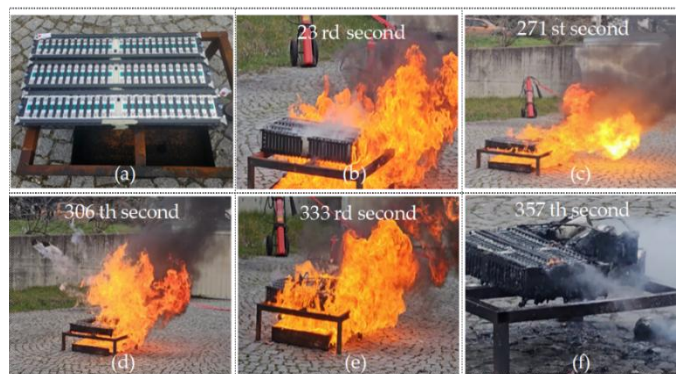
Figure 3. (a) Experiment set-up, (b) intensive white smoke, (c) first explosion, (d) cathode and anode foils extraction by an explosion, (e) LIB module frame lost its strength, LIB cells fell into the pan, and (f) LIB modules condition after extinguishing
