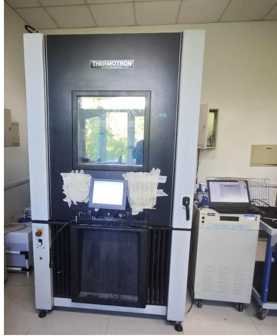
Fig.2 Photograph of the temperature-controlled chamber and data acquisition equipment
