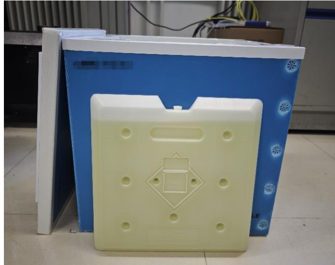
Fig.1 Photograph of the cold storage box and phase change material (PCM) packages
