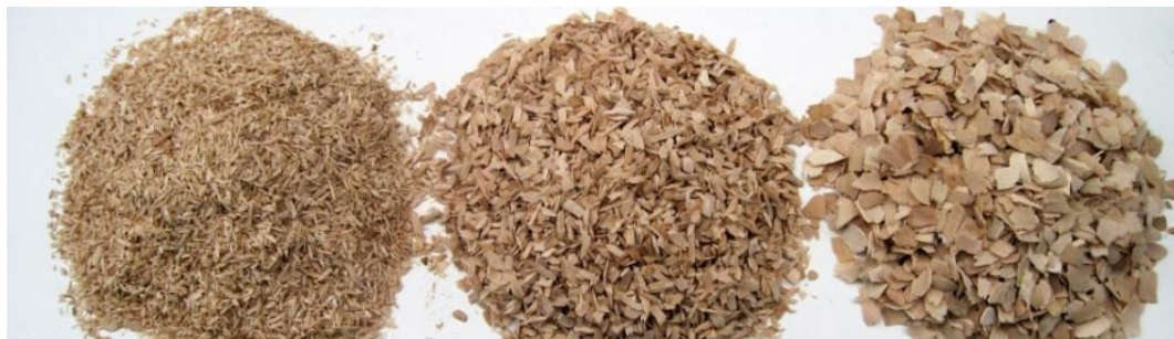
Figure 2. Sawdust as a potential component in the biobased insulation material
