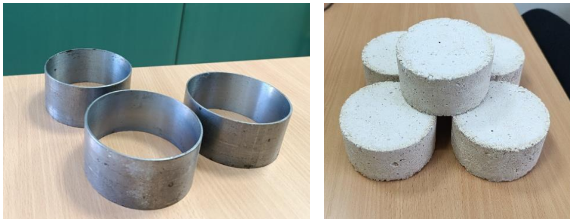
Figure 4. The mold for making the samples and the finished samples
