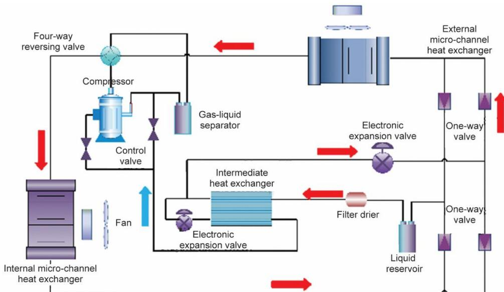
**Figure 2. System cycle principle**
