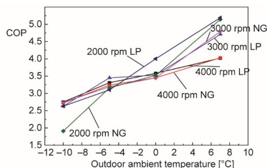
Figure 4. Outside ambient temperature impact on the system COP
