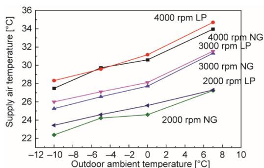
**Figure 5.** Outside ambient temperature impact on the supply air temperature
