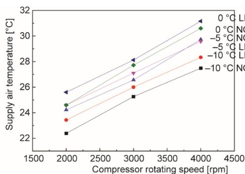
**Figure 10. Effect of compressor speed impact on the supply air temperature**
