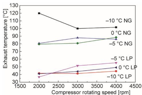
**Figure 7.** Effect of compressor speed impact on exhaust temperature
