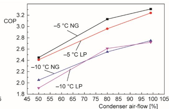
**Figure 12.** The amount of condenser air-flow impact on the system COP
