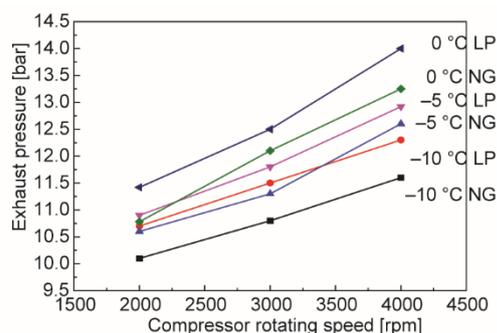
**Figure 6.** Effect of compressor speed impact on the exhaust pressure
