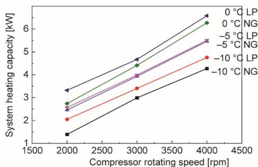
**Figure 8.** Effect of compressor speed impact on system heating capacity
