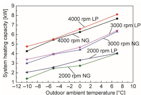
Figure 3. Outside ambient temperature impact on the system heating capacity
