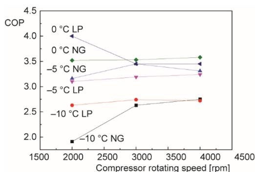
**Figure 9. Effect of compressor speed impact on the system COP**
