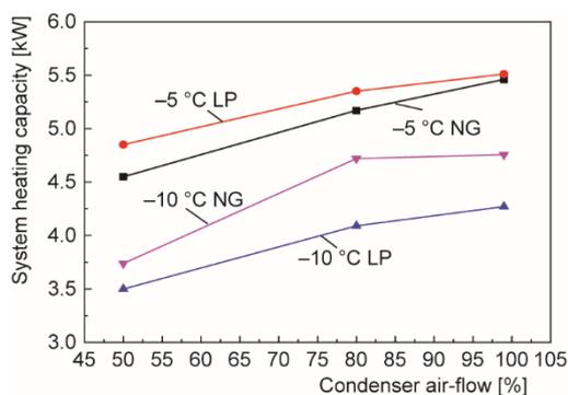
**Figure 11.** The amount of condenser air-flow impact on the heating capacity
