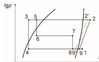
**Figure 1. Low pressure gas supplement system**
