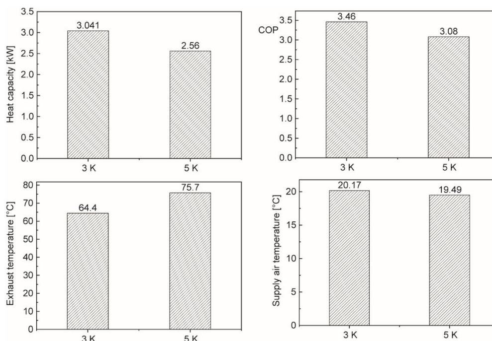
Figure 9. Impact of main valve superheat on system heating performance
