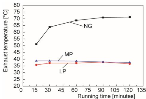
**Figure 7. Impact of gas supplementation methods on exhaust temperature**
