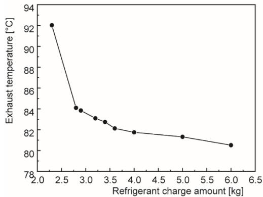
**Figure 5. Variation of exhaust temperature with amount of refrigerant**
