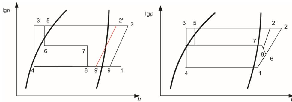
**Figure 2. Theoretical cycle of the system; (a) low pressure gas supplement theory cycle and (b) medium pressure gas supplement theory cycle**
