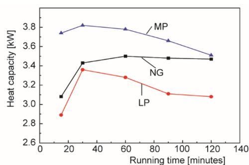
**Figure 8. Impact of gas supplementation methods on system heating capacity**
