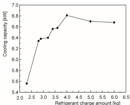
**Figure 3. Variation of cooling capacity with amount of refrigerant**
