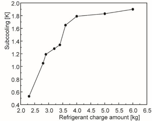
**Figure 6. Variation of sub-cooling with amount of refrigerant**
