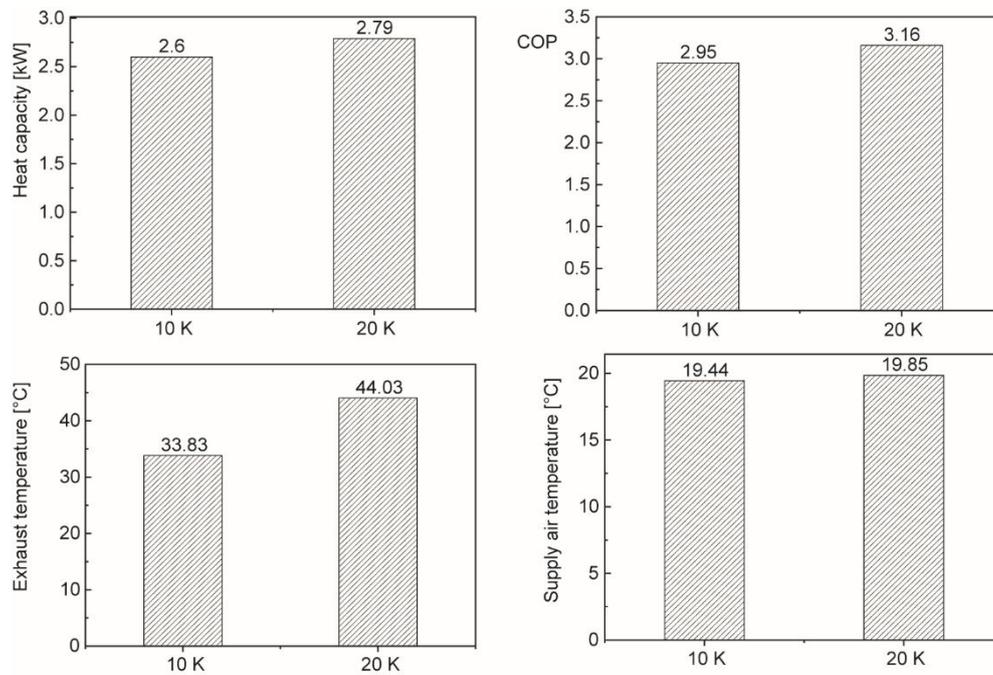
Figure 10. Impact of auxiliary valve superheat on system heating performance
