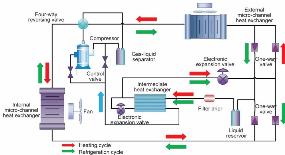
**Figure 1. System cycle principle**
