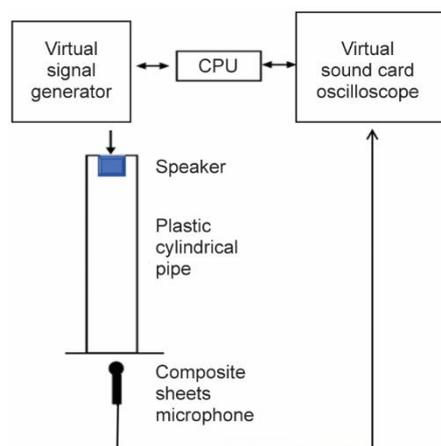
**Figure 1.** Testing device of acoustic property about composite
