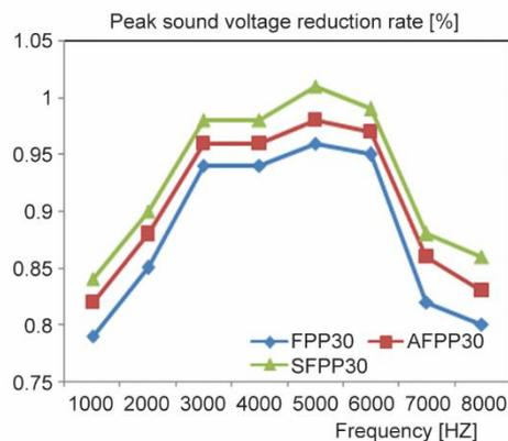
Figure 4. Effects of surface modification on acoustic property of flax/polypropylene composites
