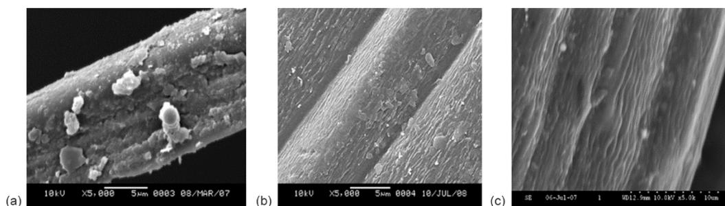
Figure 2. The SEM photographs of different modified flax fibers (a) untreated, (b) alkali treated, and (c) KH-570 treated
