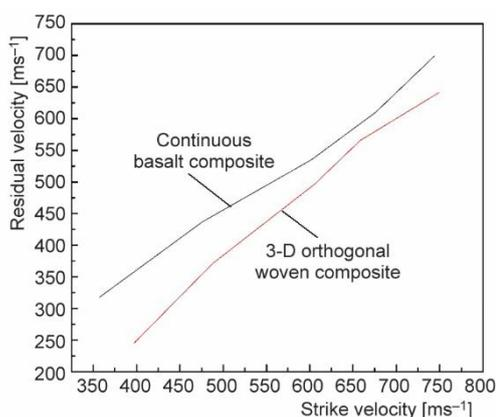
Figure 1. Velocity-residual velocity curve
