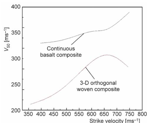
Figure 3. Ballistic limit velocity  $V_{50}$ -initial strike velocity
