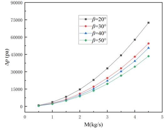
**Fig. 15. The variation of  $\Delta p$  with mass flow rate increase at different helix angles**
