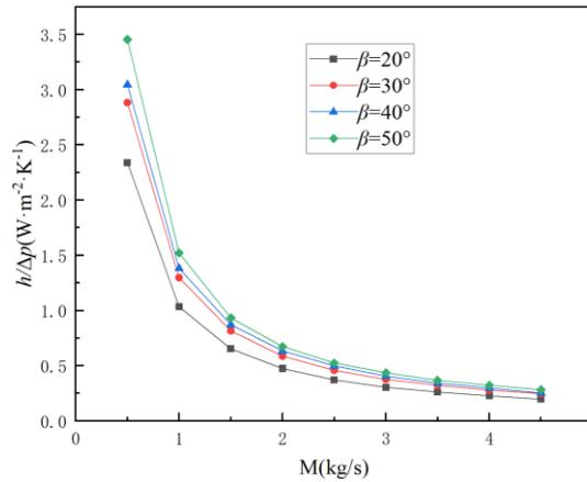
**Fig. 16. The variation of  $h/\Delta p$  with mass flow rate for different helix angles**
