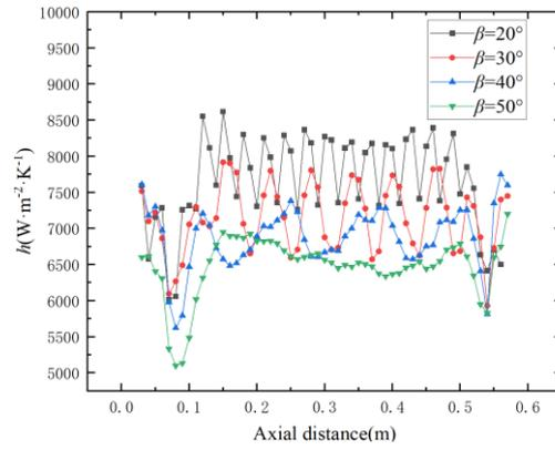
**Fig. 11. Distribution of the average surface  $h$  along the shell-side axis under different helix angles**
