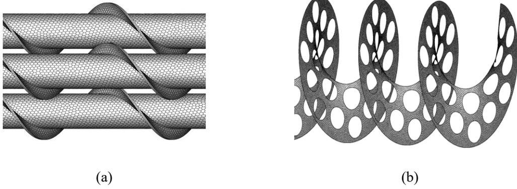
**Fig. 2. Grid of supporting structure (a) self-supporting fin tubes and (b) helical baffle**
