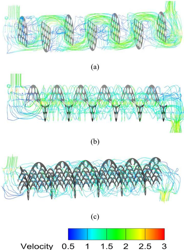
**Fig. 6. Velocity (m/s) path lines in different STHXs (a) STHX-SG and (b) STHX-HB/STHX-HBCT and (c) STHX-HBST**
