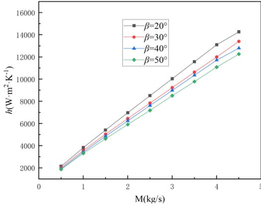
**Fig. 14. Variation of  $h$  with mass flow rate increase at different helix angles**
