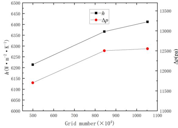
**Fig. 3. Grid independence test of STHX-HBST**
