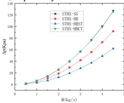
**Fig. 7. The variation of  $\Delta p$  with mass flow rate increasing**
