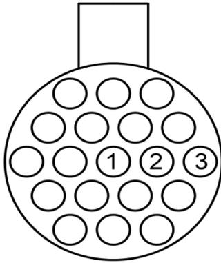
**Fig. 12. Distribution of heat exchange tubes at different radial distances**
