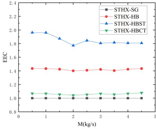
**Fig. 9. EEC with various flow rate of four STHXs**
