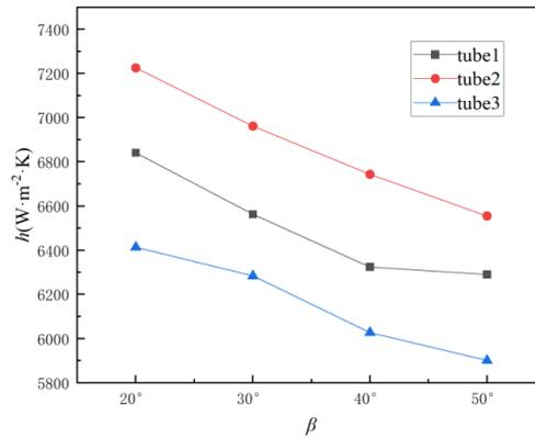
**Fig. 13.  $h$  of tubes under different helix angles.**
