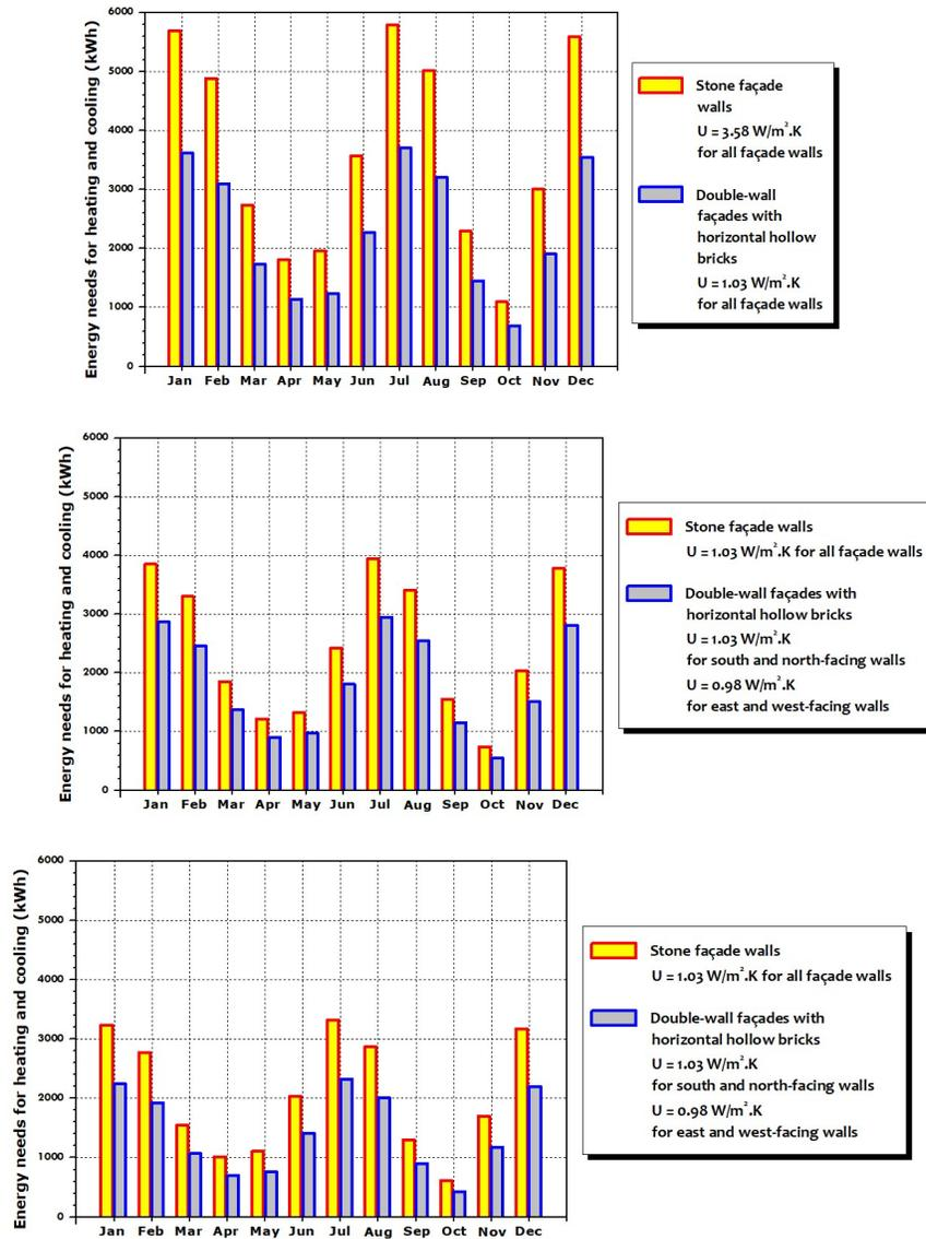
**Figure 7: Monthly energy requirements for a comfortable temperature between 21 and 26 °C, a: case of a single-story house, b: the case of east and west facing in contact with unheated areas, c: the case of high floor, east and west facing in the contact with unheated areas**
