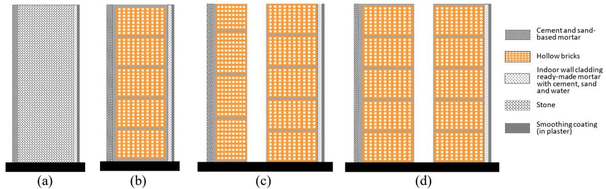
**Figure 6: House wall configuration, a: stone façade walls (reference case), b: façade walls with single hollow brick, c: double-wall façade with horizontal and vertical hollow bricks, d: double-wall façade with horizontal hollow bricks**
