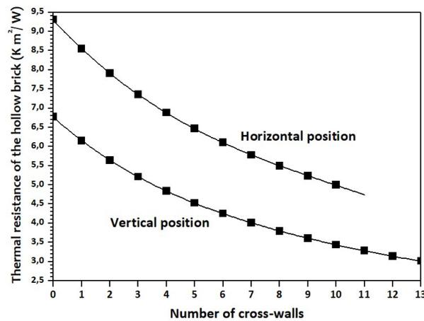
Figure 4: Variation in thermal resistance according to the number of cross-sectional walls, case of a hollow brick with 3 air cavity columns. The corresponding thickness of the air cavity is 38 mm if the brick is in the vertical position and 54.67 in the horizontal position.
