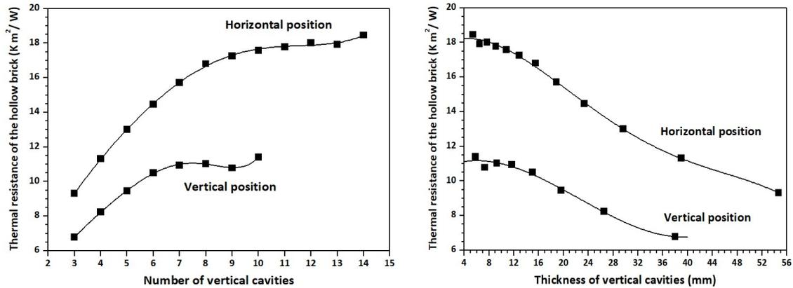
Figure 4: Variation in thermal resistance as a function of the: (a) number of air cavity columns, (b) air cavity width, case of a hollow brick without cross-sectional walls.
