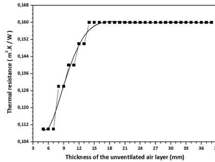
Figure 1: Thermal resistance of unventilated vertical air layers (page 23 of the reference [15])
