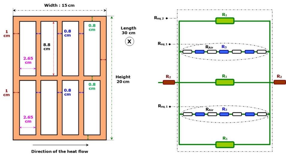
Figure 2: Geometry of the masonry unit and resistor network, case of a hollow brick with 8 identical vertical rectangular cavities of dimensions 2.65 cm x 8.8 cm
