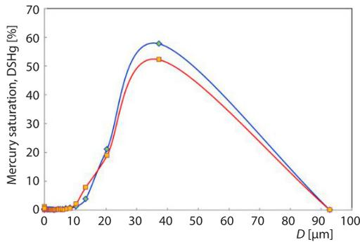
Figure 4. The relationship between pore size and mercury saturation
