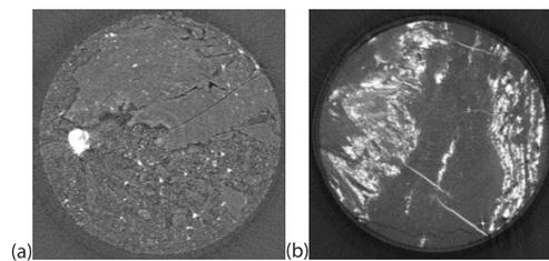
**Figure 2. The CT scan images of coal; (a) Sample-1 (25 mm) and (b) Sample-1 (2 mm)**
