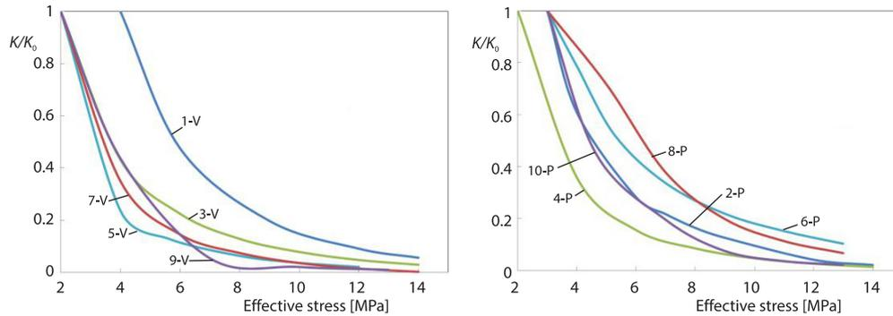
**Figure 1. The graph of dimensionless permeability variation with effective stress on vertical and parallel directions**
