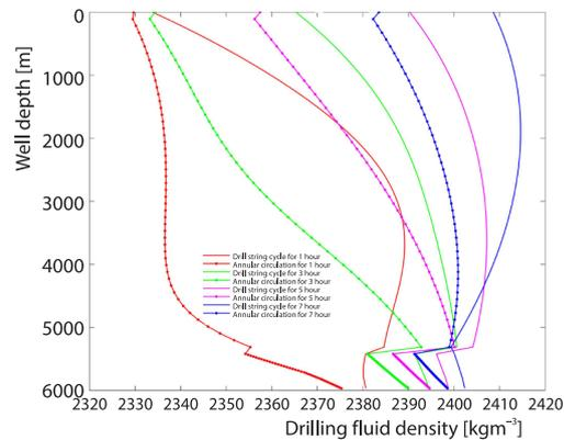
Figure 2. Density field distribution of drilling fluid
