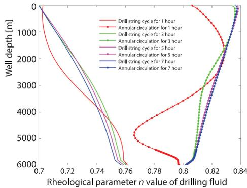
**Figure 3. Variation of  $n$  values of drilling fluid rheological parameters**
