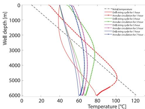
**Figure 1. Variation of circulating temperature profile in the drill string and annulus with time**
