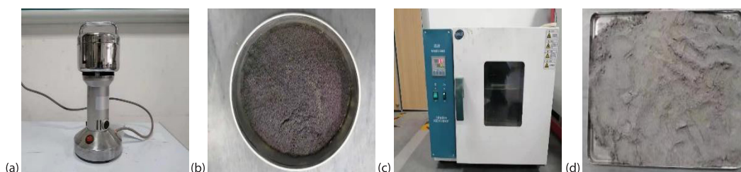
Figure 4. Pretreatment of experimental materials; (a) experimental material crushing, (b) test material sifting, (c) experimental drying material, and (d) experimental material after drying
