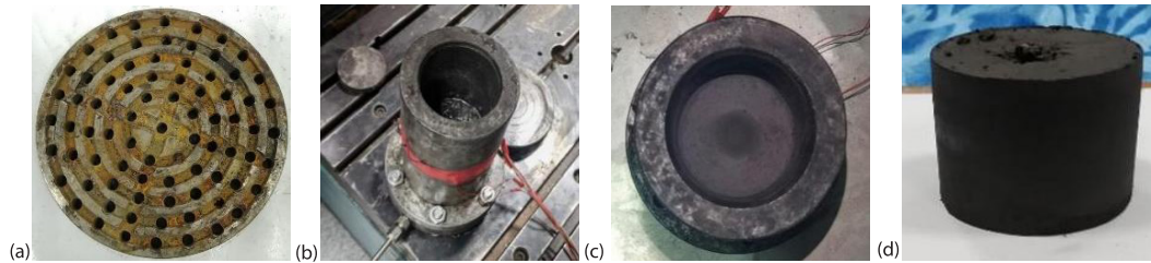
Figure 1. Compaction test flow; (a) install the permeable plate, (b) add fly ash paste, (c) compaction, and (d) remove cake
