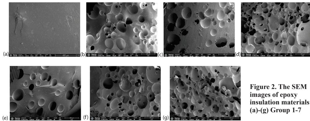
Figure 2. The SEM images of epoxy insulation materials: (a)-(g) Group 1-7
