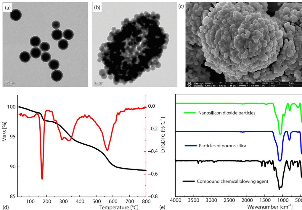
**Figure 1. Characterization results of compound blowing agent;**
