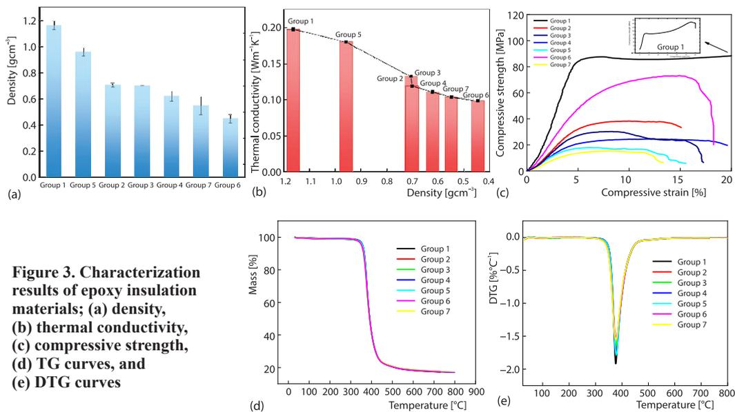
**Figure 3. Characterization results of epoxy insulation materials; (a) density, (b) thermal conductivity, (c) compressive strength, (d) TG curves, and (e) DTG curves**
