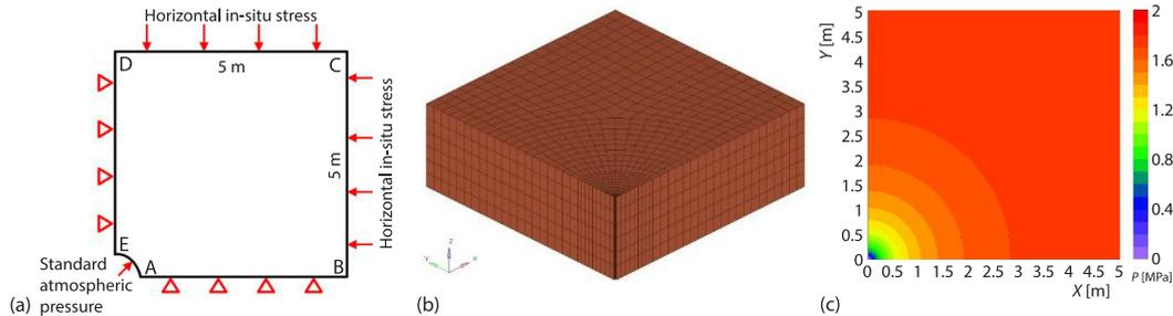
**Figure 2. Schematic diagram of 1/4 model of Xinzhuangzi coal mine; (a) schematic diagram of mechanical model, (b) grid division diagram, (c) pressure distribution in coal seam**
