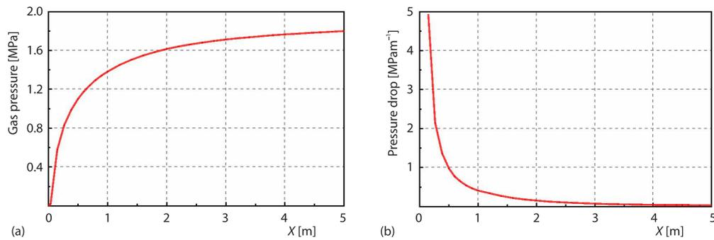
**Figure 3. The influence of drilling center distance on gas pressure (a) and gas pressure drop (b)**
