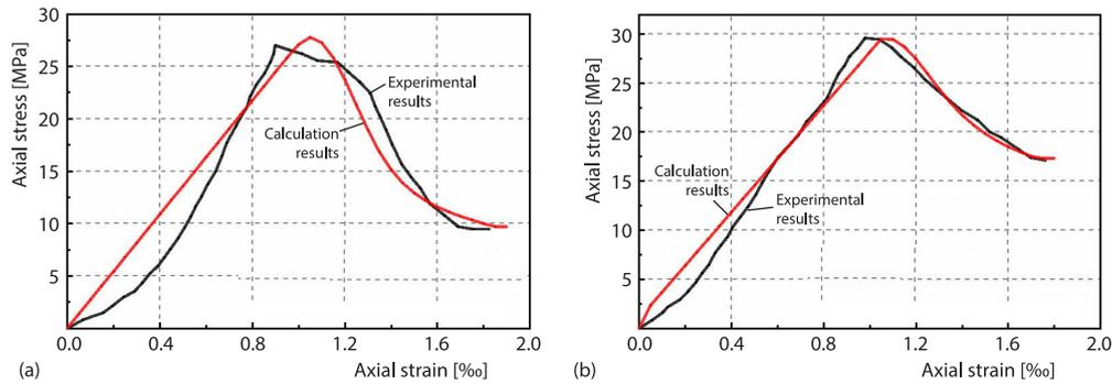
**Figure 1. Comparison of the experimental data and the calculation results of the elastoplastic damage constitutive model under various confining pressures; (a)  $P_c = 0$  MPa and (b)  $P_c = 2$  MPa**
