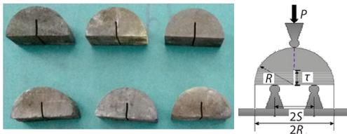
**Figure 1.** Shale specimens and their experimental loading schematic diagram
