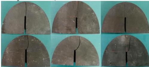
Figure 5. Fracture paths of shale before and after LN<sub>2</sub> treatment
