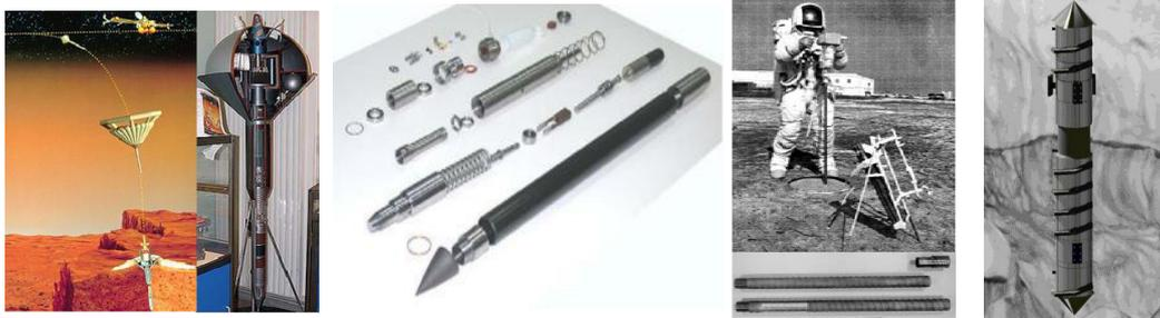
Figure 1. Extraterrestrial body sampling methods; (a) kinetic penetration, (b) impact penetration sampling, (c) spiral drilling sampling, and (d) autonomous excavation
