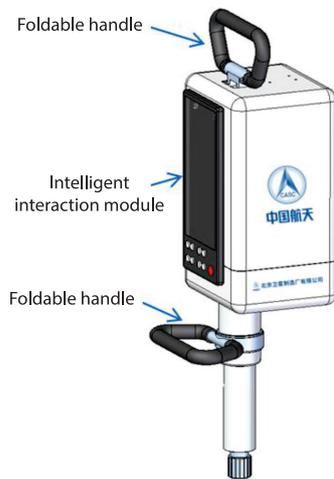
**Figure 4. Drill rig structure schematic**
