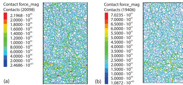
**Figure 2. Distribution characteristics of contact force between particles following PBM application under different numerical simulation processes; (a) new numerical simulation process and (b) traditional numerical simulation process**
