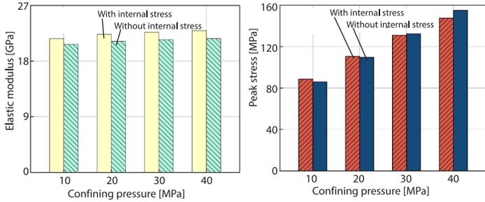
**Figure 4.** Comparison of mechanical parameters with and without internal stress; (a) elastic modulus and (b) peak stress
