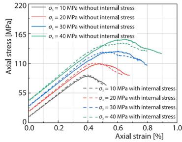
**Figure 3.** Changes in stress-strain curve with and without internal stress
