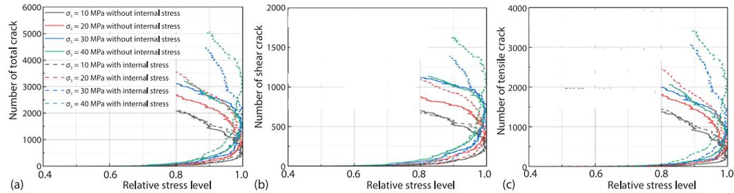
**Figure 5.** Changes in the number of cracks in the rock numerical model with and without internal stress during the loading process; (a) total crack, (b) shear crack, and (c) tensile crack
