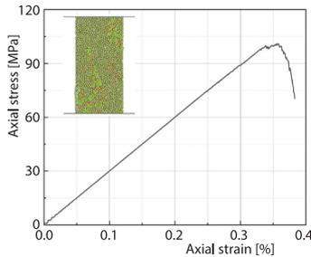
**Figure 1. Calibration results of uniaxial compression test based on PFC2D**
