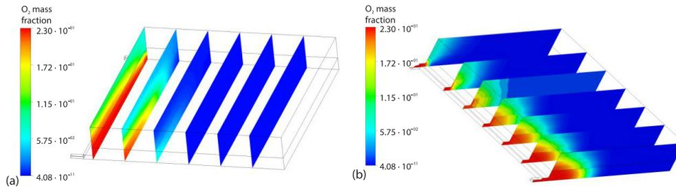
**Figure 5. Cross-sectional contours of O<sub>2</sub> mass fraction distribution in the goaf; (a) overall *X* cross-sectional contour map and (b) overall *Y* cross-sectional contour map**
