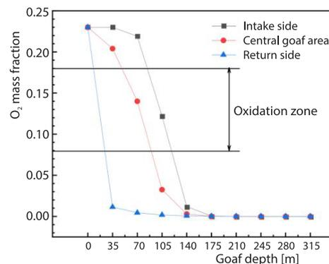
Figure 4. Variation of  $O_2$  mass fraction on the intake, return sides, and middle of the goaf
