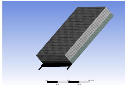
Figure 2. Meshing diagram of the goaf
