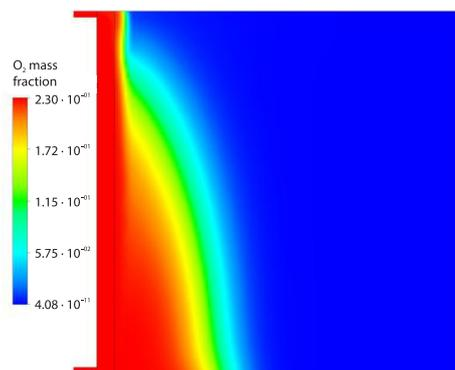
Figure 3. The  $O_2$  mass fraction distribution in the goaf
