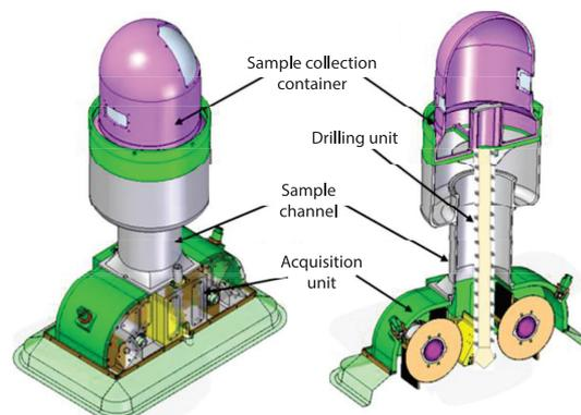
Figure 5. Composite asteroid sampling system
