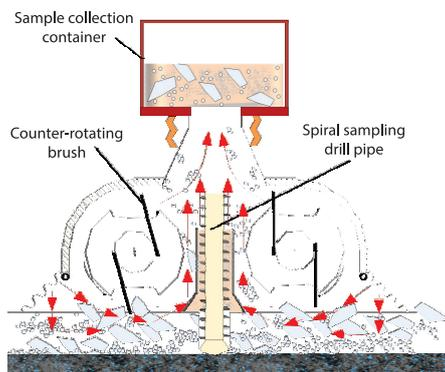
Figure 4. Compound sampling principle
