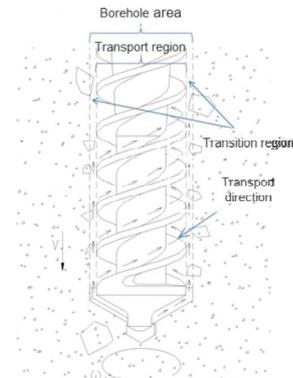
Figure 3. Drilling transport sampling
