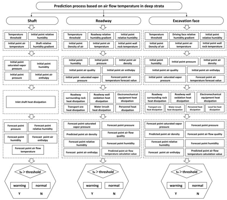
Figure 2. Prediction skeleton based on air-flow temperature in deep strata
