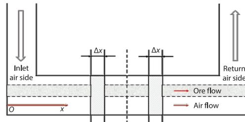
Figure 1. Geometric model of air-flow temperature prediction in deep strata
