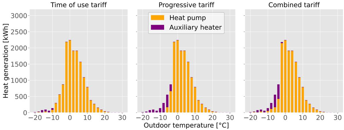
**Figure 7. Dependence of the annual heat demand coverage on the outdoor temperature**
