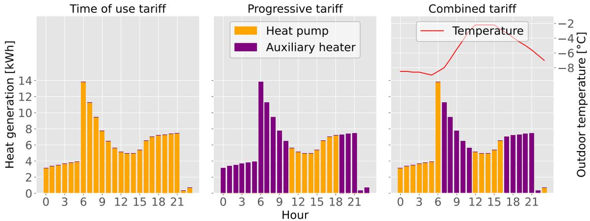
Figure 6. Example of daily heat pump and auxiliary heater scheduling
