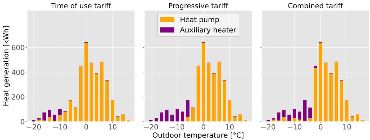
**Figure 8. Dependence of the monthly heat demand coverage on the outdoor temperature**
