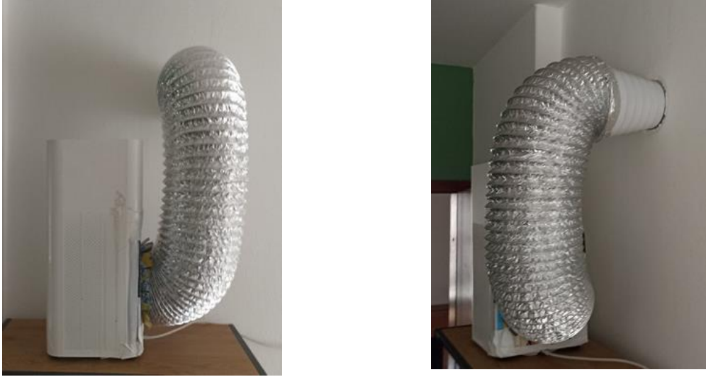
Figure 2. The modified Xiaomi Mi 2H air purifier: front and side view
