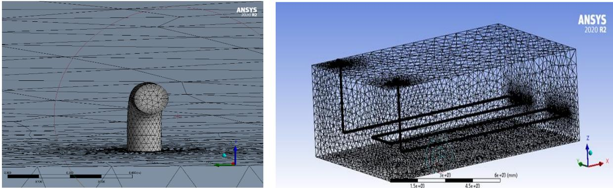
a) Three-dimensional view of air inlet and outlet. b) Three-dimensional view of earth-air heat exchanger.
