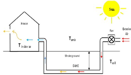
Figure 1. Earth air heat exchanger.
