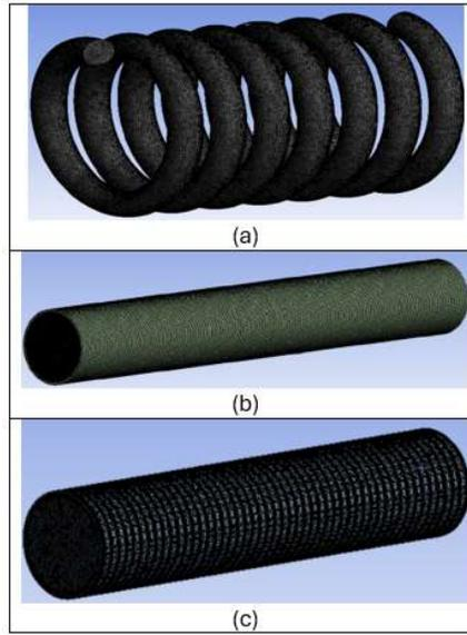
**Figure 2. Appearances of pipe mesh structures; a) Helical, b) Corrugated, c) Dimpled**
