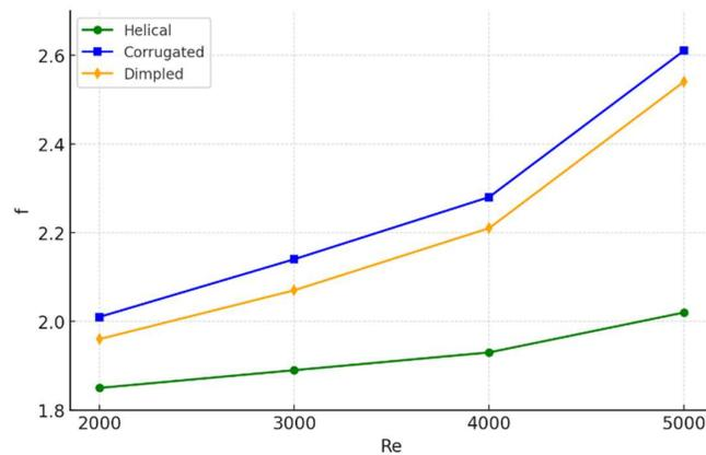
**Figure 4. Comparison of skin friction coefficient values of different pipe designs according to Reynolds number**
