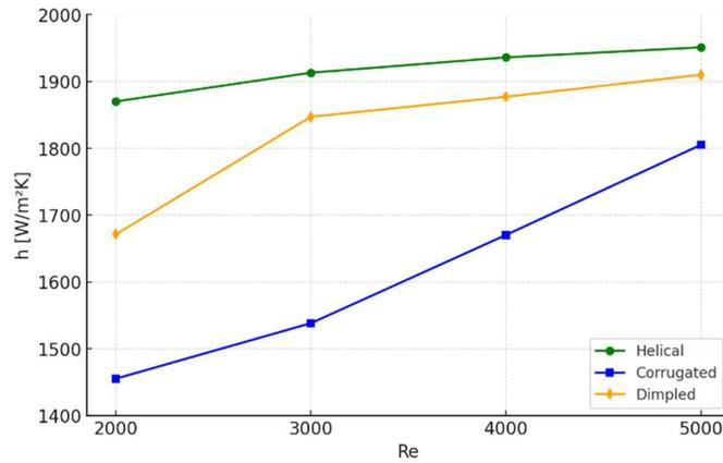
**Figure 3. Comparison of heat transfer coefficients of different pipe designs according to Reynolds number**
