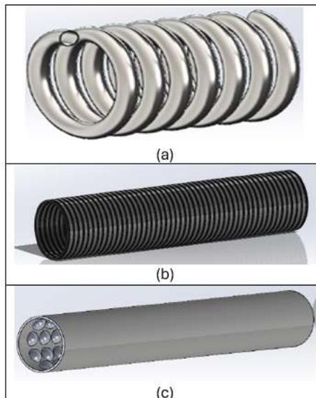
**Figure 1. Appearances of designed pipes; a) Helical, b) Corrugated, c) Dimpled**
