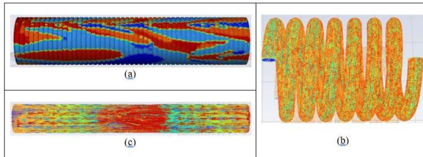
**Figure 6. Temperature contours calculated by the  $k-\omega$  SST turbulence model at  $Re = 2000$ : (a) corrugated pipe, (b) helical pipe, (c) dimpled pipe**
