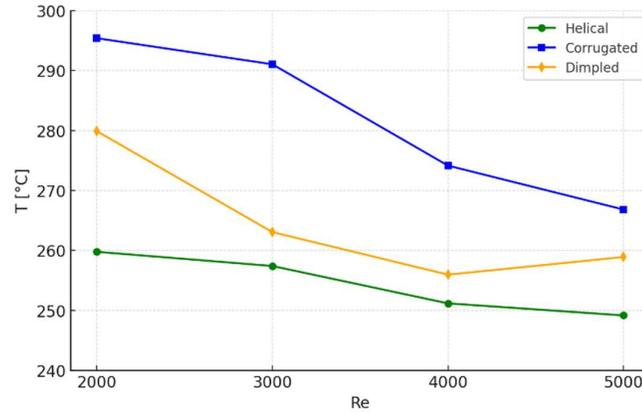
**Figure 5. Comparison of maximum wall temperature values of different pipe designs according to Reynolds number**
