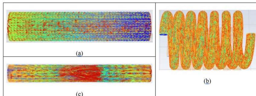
**Figure 7. Temperature contours calculated by the  $k-\omega$  SST turbulence model at  $Re = 5000$ : (a) corrugated pipe, (b) helical pipe, (c) dimpled pipe**
