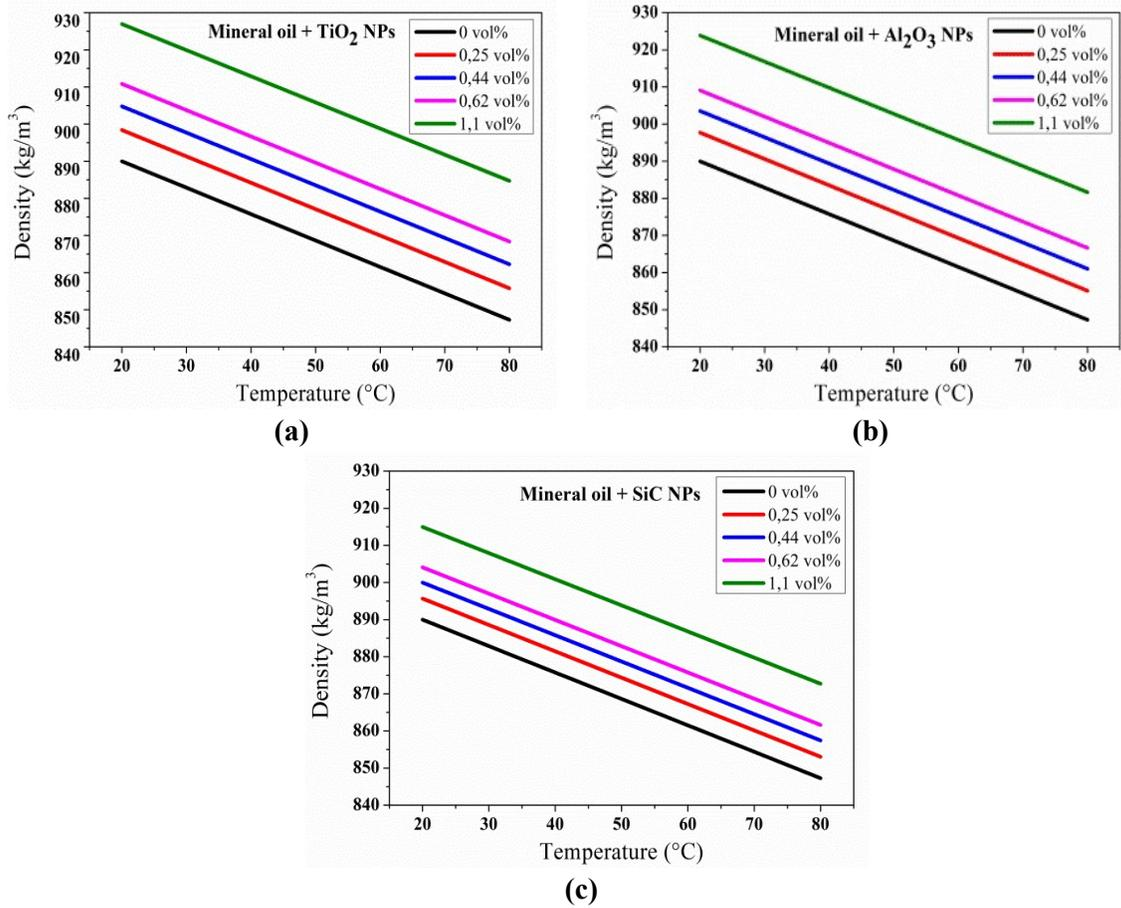
**Figure 7. Density of pure dielectric oil and dielectric nanofluids: (a) MO + TiO<sub>2</sub> NPs; (b) MO + Al<sub>2</sub>O<sub>3</sub> NPs; (c) MO + SiC NPs**
