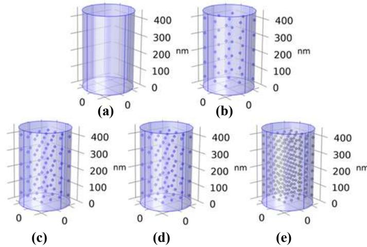
**Figure 2. Geometry of model after applying different concentrations of nanoparticles in the dielectric fluid: (a) MO + 0 vol% NPs; (b) MO + 0.25 vol% NPs; (c) MO + 0.44 vol% NPs; (d) MO + 0.62 vol% NPs; (e) MO + 1.1 vol% NPs**
