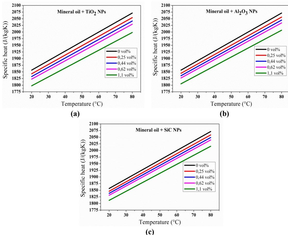
**Figure 6. Specific heat of pure dielectric oil and dielectric nanofluids: (a) MO + TiO<sub>2</sub> NPs; (b) MO + Al<sub>2</sub>O<sub>3</sub> NPs; (c) MO + SiC NPs**
