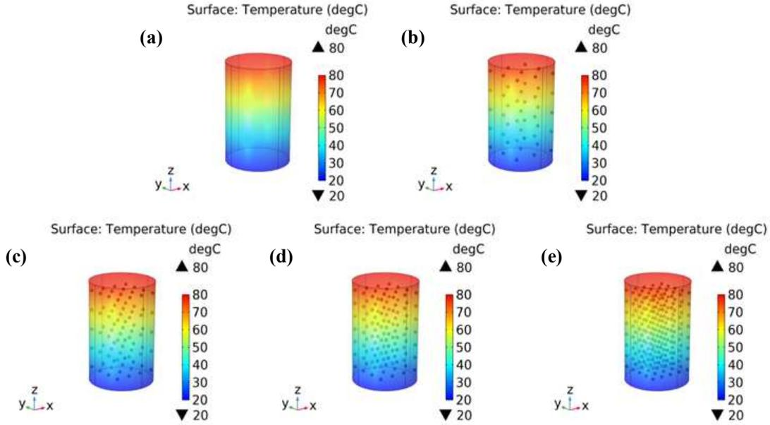
**Figure 3. The studied model after applying a temperature gradient: (a) MO + 0 vol% NPs; (b) MO + 0.25 vol% NPs; (c) MO + 0.44 vol% NPs; (d) MO + 0.62 vol% NPs; (e) MO + 1.1 vol% NPs**
