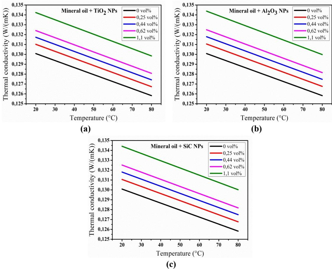
**Figure 4. Thermal conductivity of pure dielectric oil and dielectric nanofluids: (a) MO + TiO<sub>2</sub> NPs; (b) MO + Al<sub>2</sub>O<sub>3</sub> NPs; (c) MO + SiC NPs**
