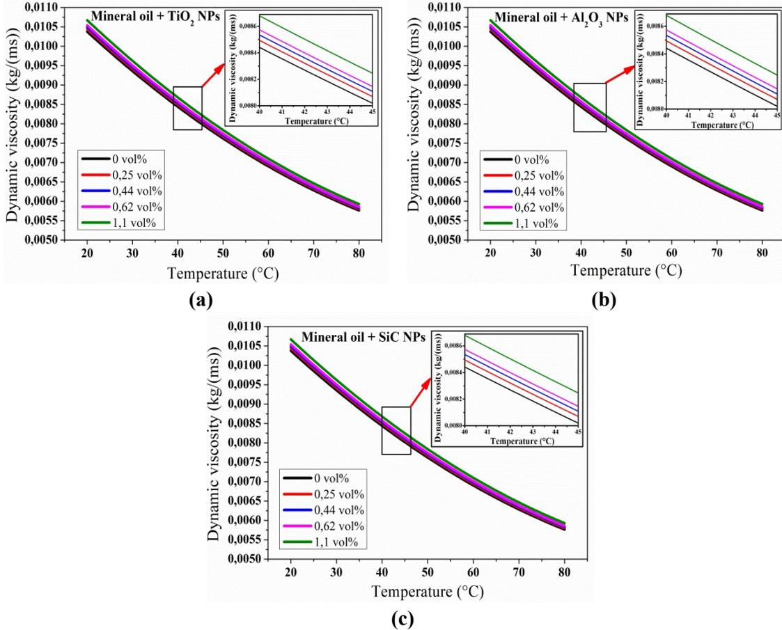
**Figure 5. Viscosity of pure dielectric oil and dielectric nanofluids: (a) MO + TiO<sub>2</sub> NPs; (b) MO + Al<sub>2</sub>O<sub>3</sub> NPs; (c) MO + SiC NPs**
