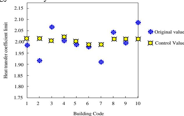
Fig. 1 Average heat transfer control results of consumption prefabricated building exterior walls
