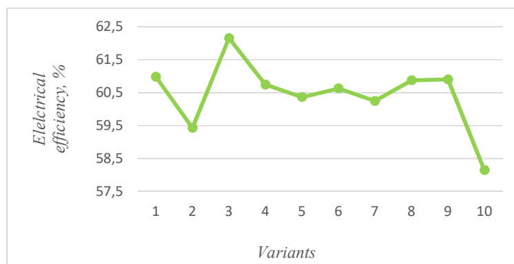
Figure 9. Efficiency of the system at the different variants of synthesis gas composition.
