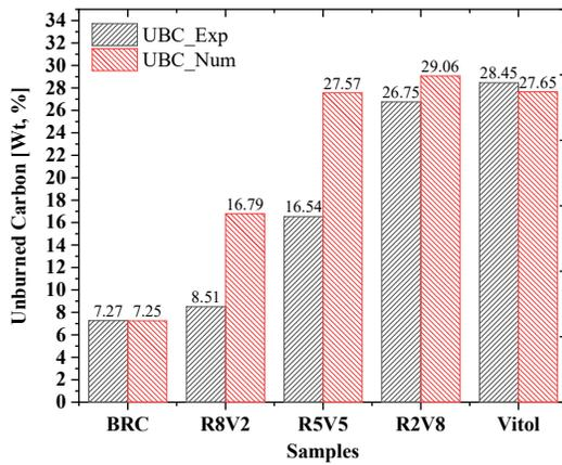
c) UBC of mixture BRC and Vitol
