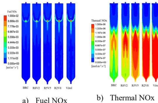
**Fig. 8. Distributions of NO<sub>x</sub> formation rates of mixture of BRC and Vitol**
