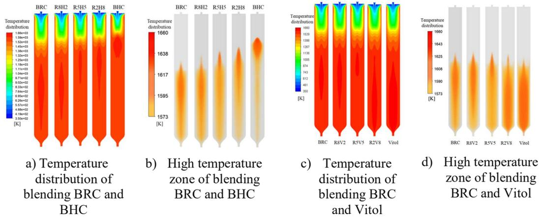
**Fig. 5. Temperature distribution in vertical cross section**
