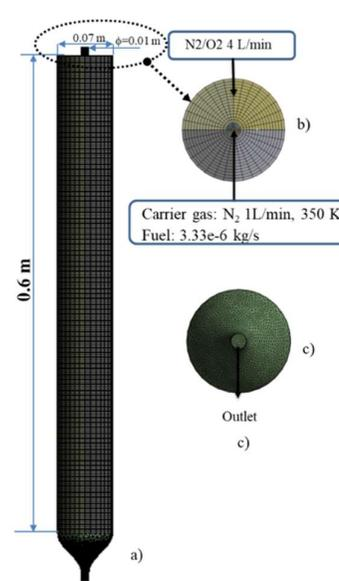
**Fig. 2. Geometry and mesh of DTF: (a) Front view (b) Top view (c) Bottom view**
