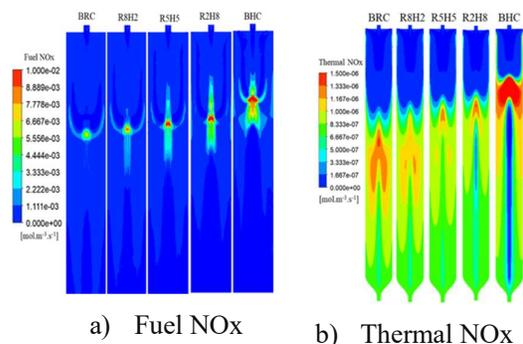
**Fig. 7. Distributions of NO<sub>x</sub> formation rates of mixture of BRC and BHC**
