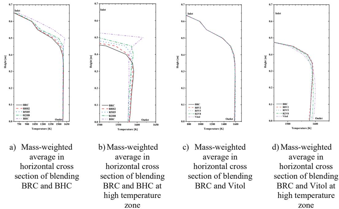
**Fig. 6. Average temperature distribution in vertical cross section**
