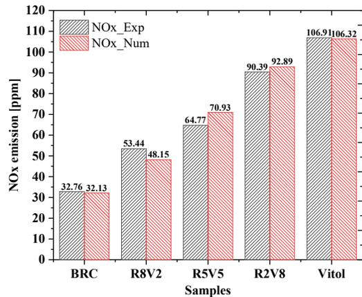
d) NOx emission of mixture BRC and BHC
