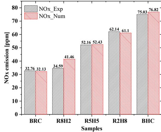
b) NOx emission of mixture BRC and BHC
