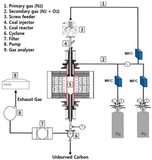
**Fig. 1. Schematic diagram of DTF test equipment**
