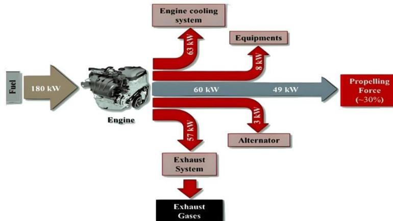
**Figure 1. Distribution of energy obtained from fuel in the engine.**
