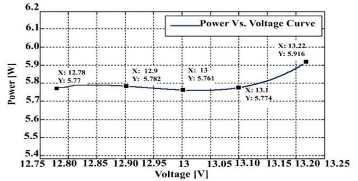
**Figure 7.(a) Relationship between Peltier voltage and current, (b) Relationship between generated power and voltage.**
