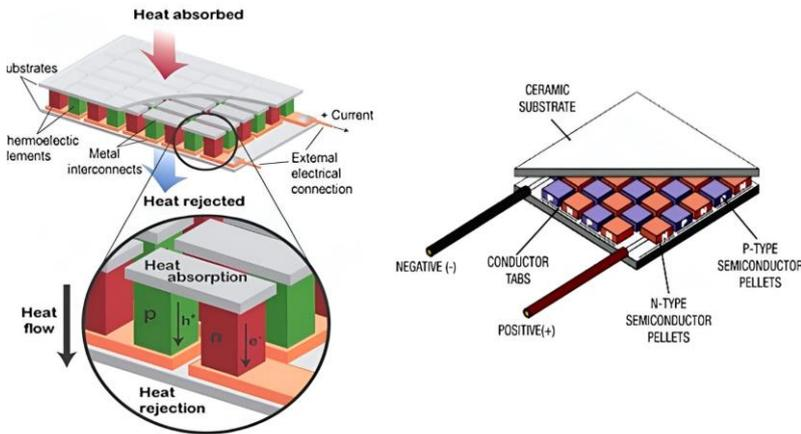
**Figure 2. Schematic representation of p–n junctions in TEG devices**
