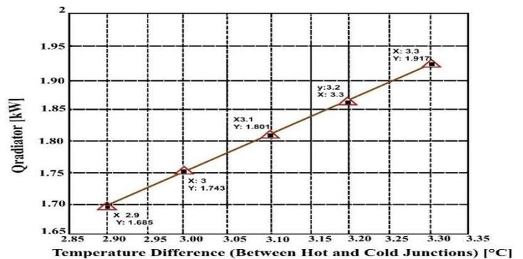
**Figure 8. (a) Relationship between generated power and current, (b) Relationship between radiator heat load  $Q_{radiator}$  and the temperature difference between radiator inlet and outlet**
