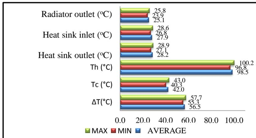
**Figure 6. Radiator outlet temperature, heat sink inlet/outlet temperatures,  $T_h$ ,  $T_c$  and temperature difference  $\Delta T$  data logger are analyzed.**
