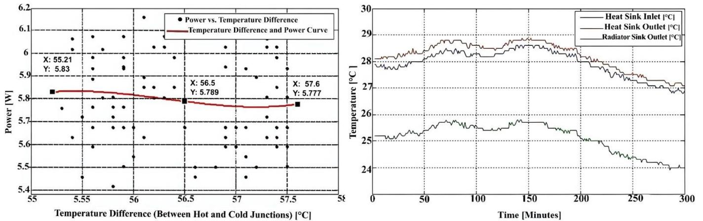
**Figure 5.(a) Temperature difference between the hot and cold junctions and corresponding power production; (b) Coolant temperature variations.**
