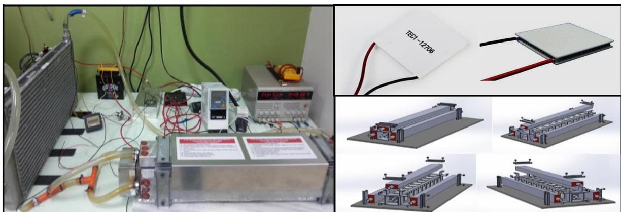
**Figure 3. General view of the experimental setup, including a detailed view of the TEC 12706 module and the exhaust pipe with cooling blocks.**
