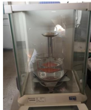
Figure 9. Hydrostatic balance of measuring porosity
