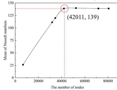
**Fig. 3 Grid independence verification results**
