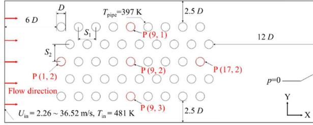
**Fig. 1 Geometric model diagram**
