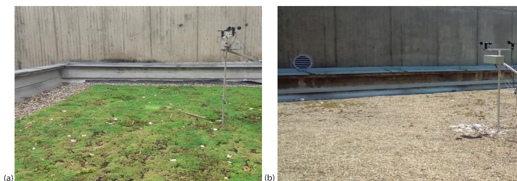
Figure 2. (a) The extensive green roof and (b) reference roof with monitoring sensors
