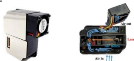
Figure 3. The particulate matter PMS3003 sensor
