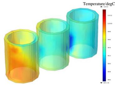
**Figure 4 (d). Temperature distribution of high voltage winding**
