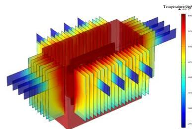
**Figure 16 (b). Transformer temperature distribution**
