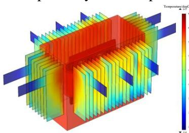
**Figure 12 (a). Overall temperature distribution of the transformer when the cooling module is installed in the upper part**
