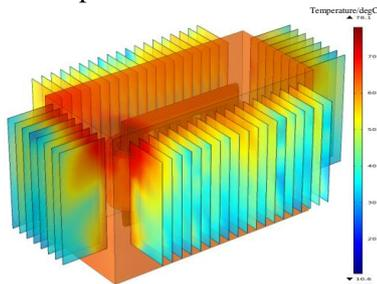
**Figure 10 (a). Temperature distribution of transformer without cooling module**
