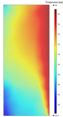
**Figure 11 (b). The temperature distribution of the heat sink without the cooling module**
