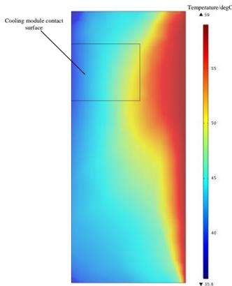
**Figure 11 (a). Temperature distribution of the heat sink for installing a cooling module**
