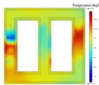
**Figure 4 (b). Temperature distribution of iron core**
