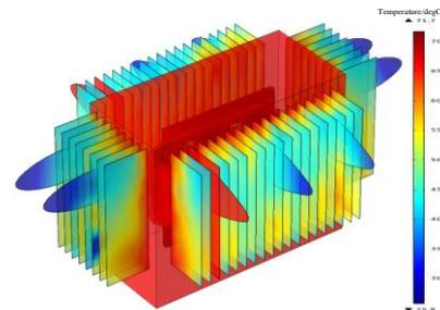
**Figure 10 (d). Overall temperature distribution of transformer when cooling module is fin**
