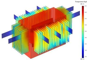
**Figure 13 (a). Overall temperature distribution of transformer when cooling module is installed symmetrically**
