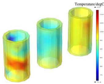
**Figure 4 (c). Temperature distribution of low voltage winding**
