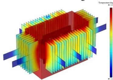
**Figure 12 (b). Overall temperature distribution of the transformer when the cooling module is installed in the middle**
