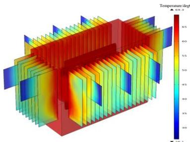
**Figure 10 (c). Overall temperature distribution of transformer when cooling module is square**
