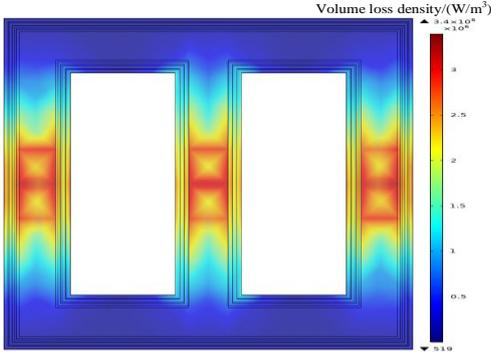
**Figure 2. Loss Density Distribution of Core**
