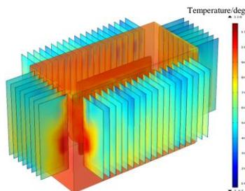
**Figure 4 (a). Temperature distribution of integral transformer**
