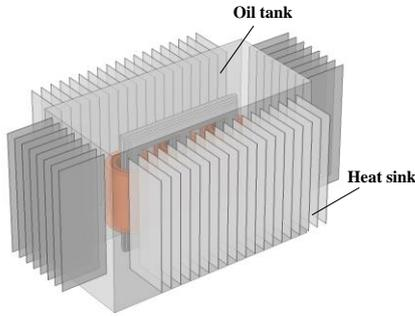
**Figure 1 (a). Three Dimensional Equivalent Model of Transformer**
