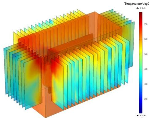
**Figure 7. Overall Temperature Distribution of Transformer after Windings Optimization**
