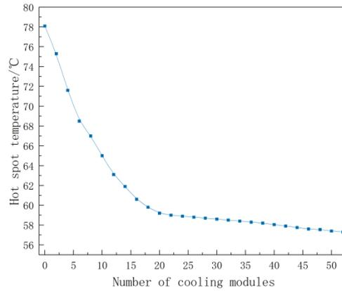
**Figure 15. Trend of Transformer Hot Spot Temperature Change**
