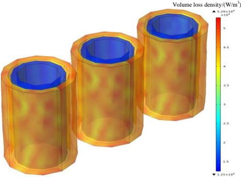
**Figure 3. Loss Density Distribution of Windings**
