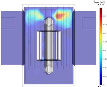
**Figure 14. Oil velocity distribution in transformer section**
