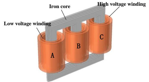
**Figure 1 (b). Internal Structure of Transformer**
