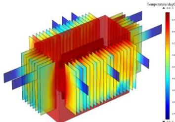
**Figure 13 (b). Overall temperature distribution of the transformer when cooling module is installed asymmetrically**
