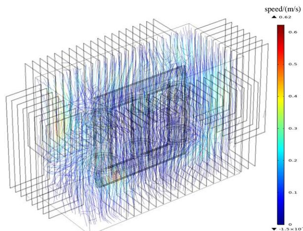
**Figure 5. Flow Distribution of Transformer**
