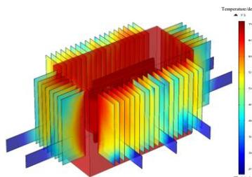
**Figure 12 (c). Overall temperature distribution of the transformer when the cooling module is installed at the lower part**
