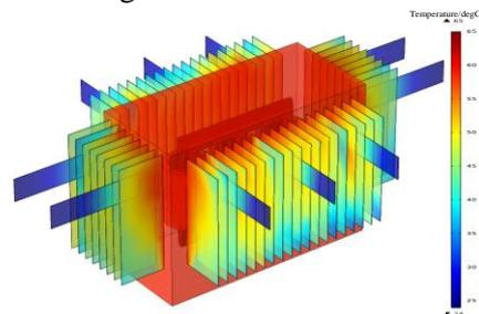
**Figure 10 (b). Overall temperature distribution of transformer when the cooling module is rectangular**
