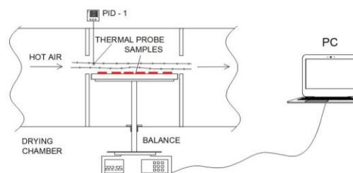
**Figure 1. Schematic drawing of drying chamber**
