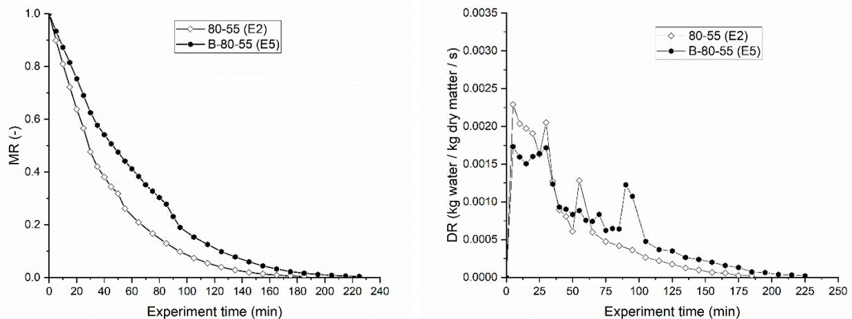
**Figure 4. Two-stages drying MR-time curve (left) and Drying rate curve (right) for blanched and untreated samples**
