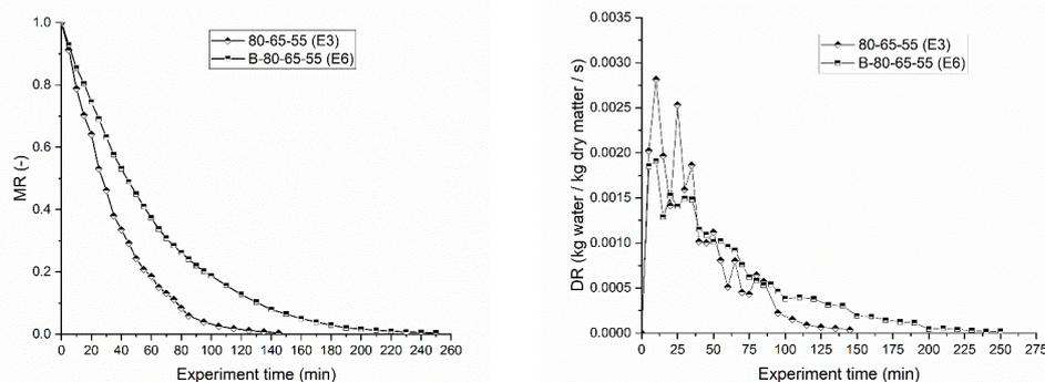
**Figure 5. Three-stage drying (with and without blanching) MR-time curve (left) and DR curve (right)**
