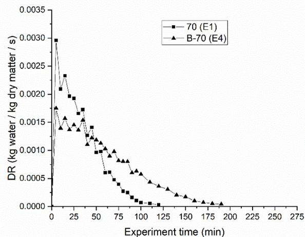
**Figure 3. Drying rate of one-stage drying of blanched (70B) and untreated sample (70)**
