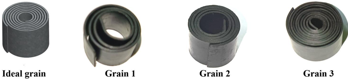
Figure 3. Spiral-shaped propellant ideal geometry and manufactured samples
