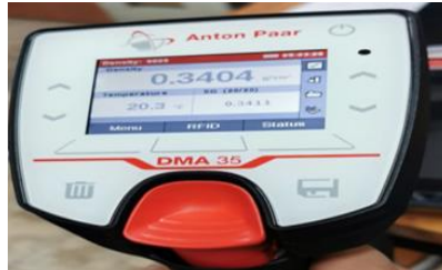
Figure 3. Anton Paar DMA 35 Densimeter, LTE laboratory/ENPO-MA.
