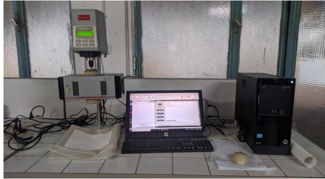
Figure 6. Anton Paar RheolabQC Viscosimeter, LTE laboratory/ENPO-MA.
