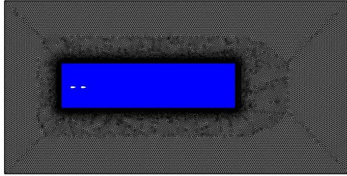
Fig.3 The mesh areas of computational domain(The blue region represents mesh1.)
