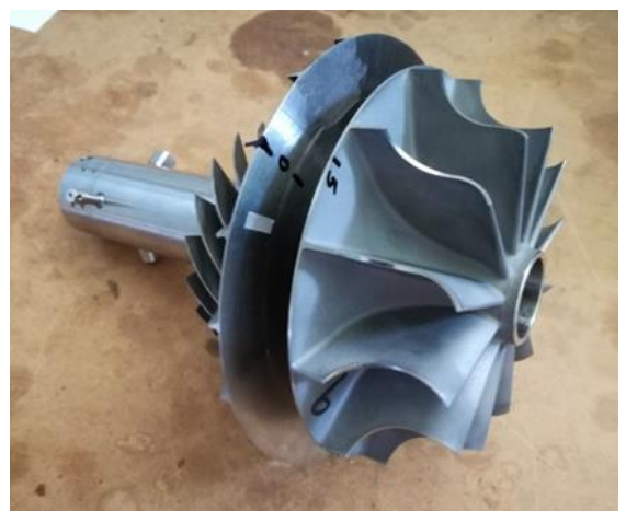
Fig. 1 – Turbo-shaft engine TSE-200 Phoenix on the left and its rotor with compressor and turbine on the right
