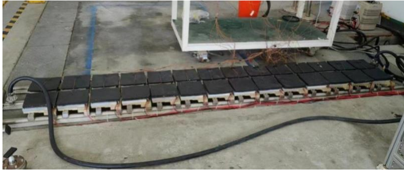
Fig. 4. Schematic of the 2 \times 7 Z-type parallel multi-branch pipe
