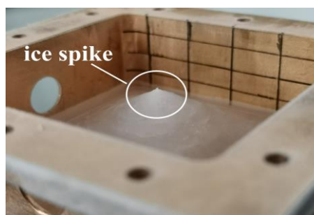
(b) Ice spike in the test cavity [35]
