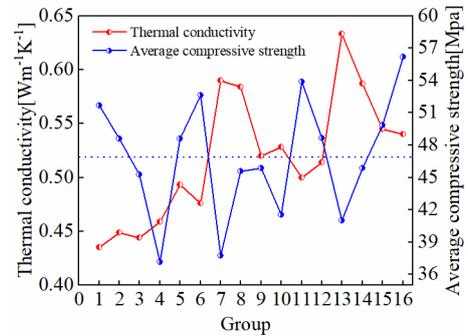
**Figure 7. Thermal conductivity and compressive strength test results**
