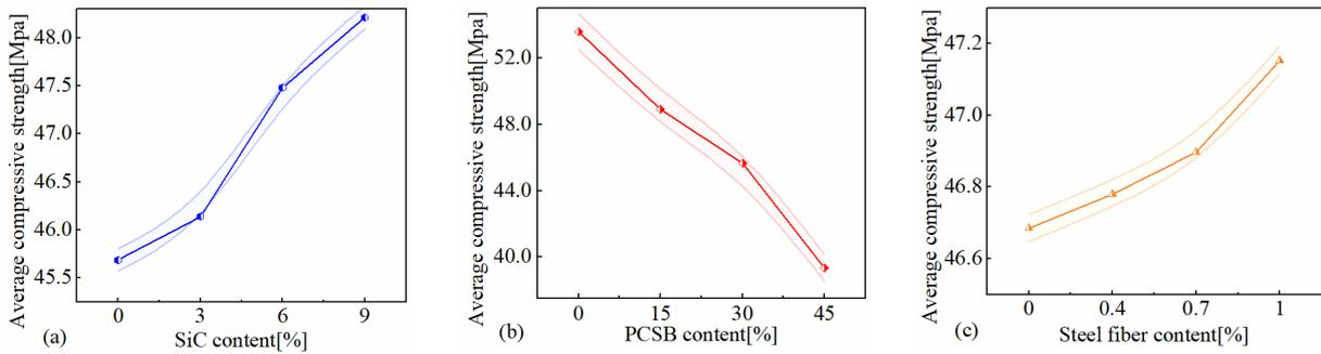
impact the compressive strength of concrete specimens. A slight strength increase is observed from 0% to 0.4%, reaching 46.79 MPa, further rising to 46.90 MPa at 0.7% dosage, and peaking at 47.15 MPa at 1% dosage. This outcome indicates that an adequate amount of steel fibers can restrict crack propagation, enhancing compressive strength.
