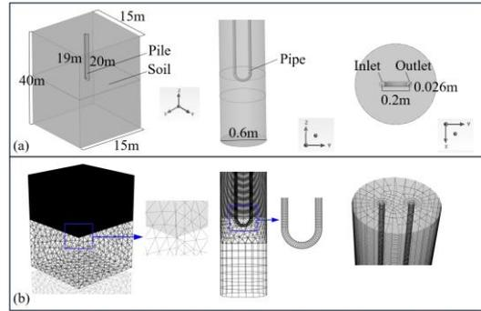
**Figure 8. Heat transfer simulation pretreatment (a) Physical model,(b) Meshing fraction**
