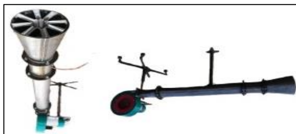
Figure 9. Experimental test bench for burner devices
