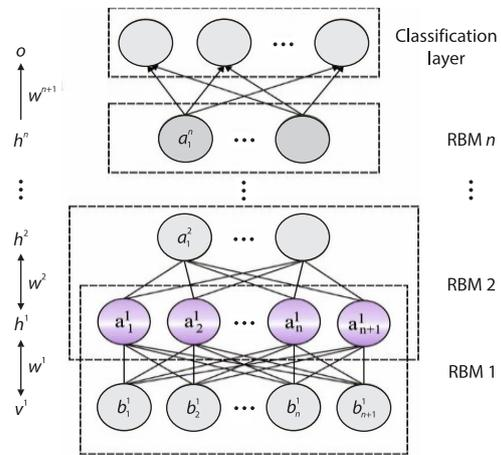
Figure 2. Structure of DBN model
