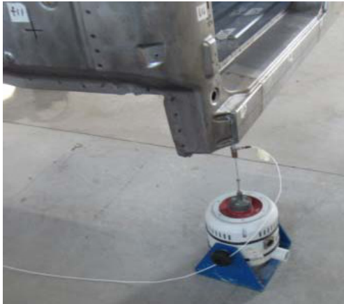
Figure 4. Reconfiguration of Shaker 1 for Installation
