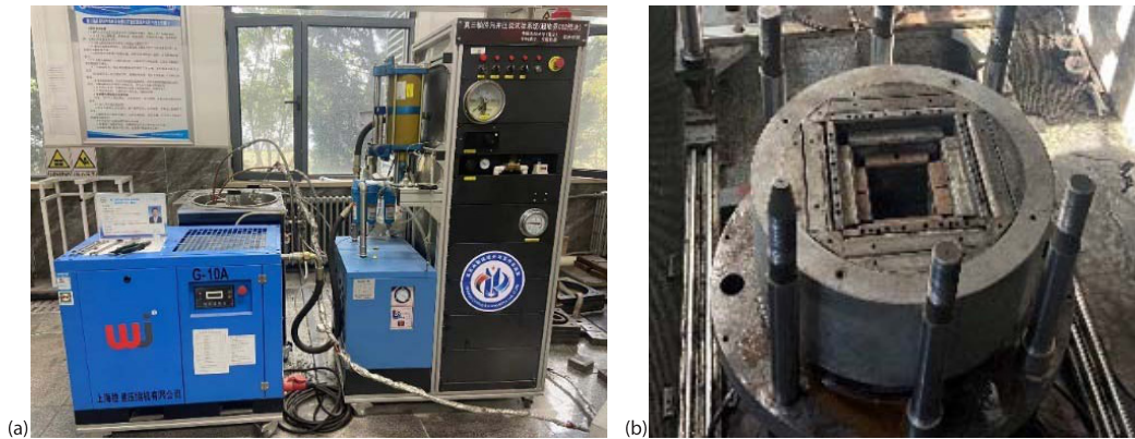
Figure 2. The SC-CO 2 fracturing experiment system; (a) SC-CO 2 supercharging device and (b) true triaxial fracturing device
