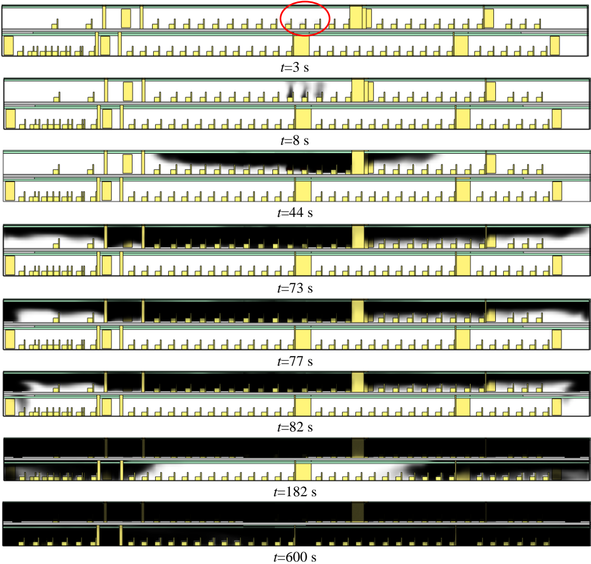
Figure 4. Spread process of cabin smoke at different times
